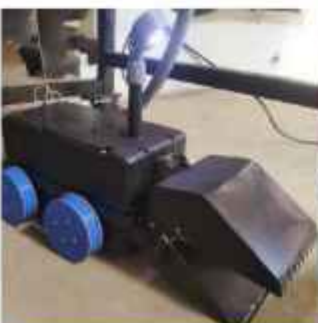
PIPE BOT FOR CLEANING
